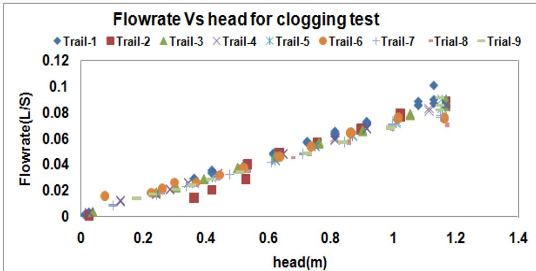
Figure 6, flowrate plotted as a function of head of water in the tank with an influent concentration increase from trial-1 to trial-9.
