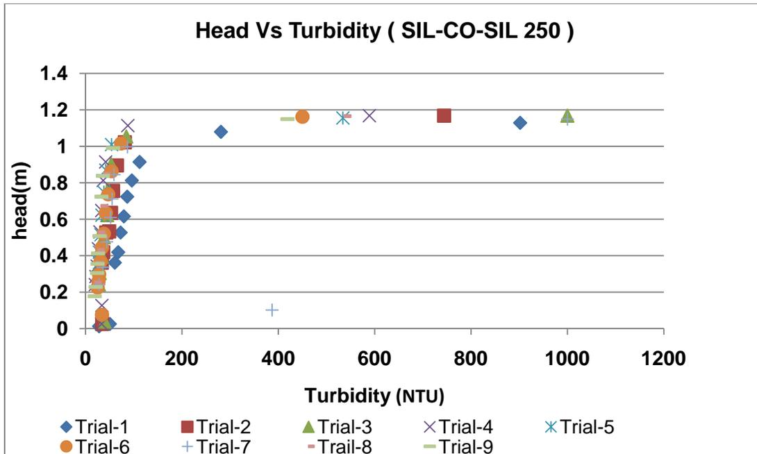
Figure 7, Turbidity as a function of head for the high purity silica (SIL-CO-SIL® 250) with increase in influent concentration at each trial.
