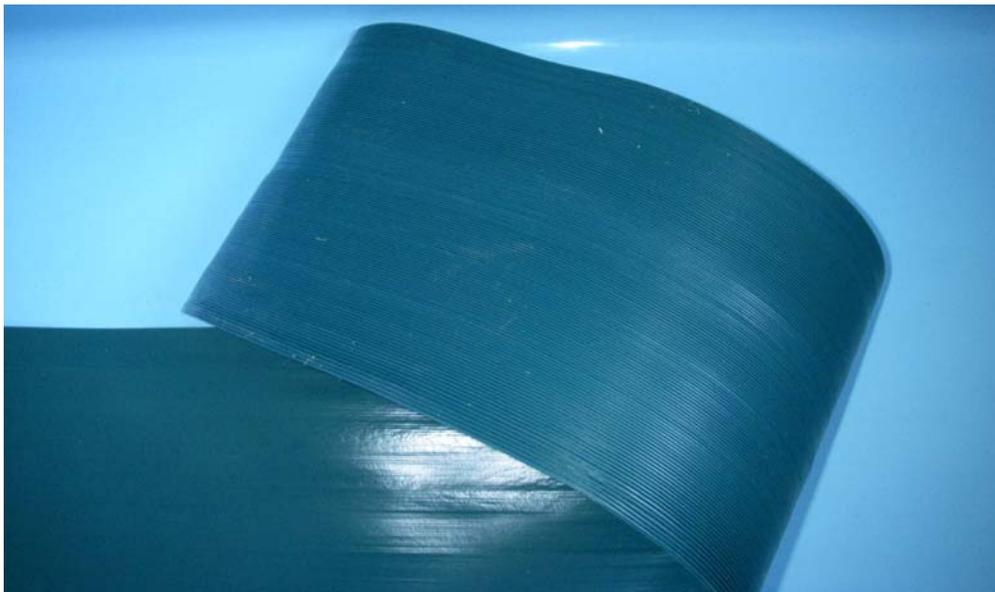
Figure 1. Close-up photograph of SmartDrain™ material showing the microchannels on the underside of the 8 in wide strip.
