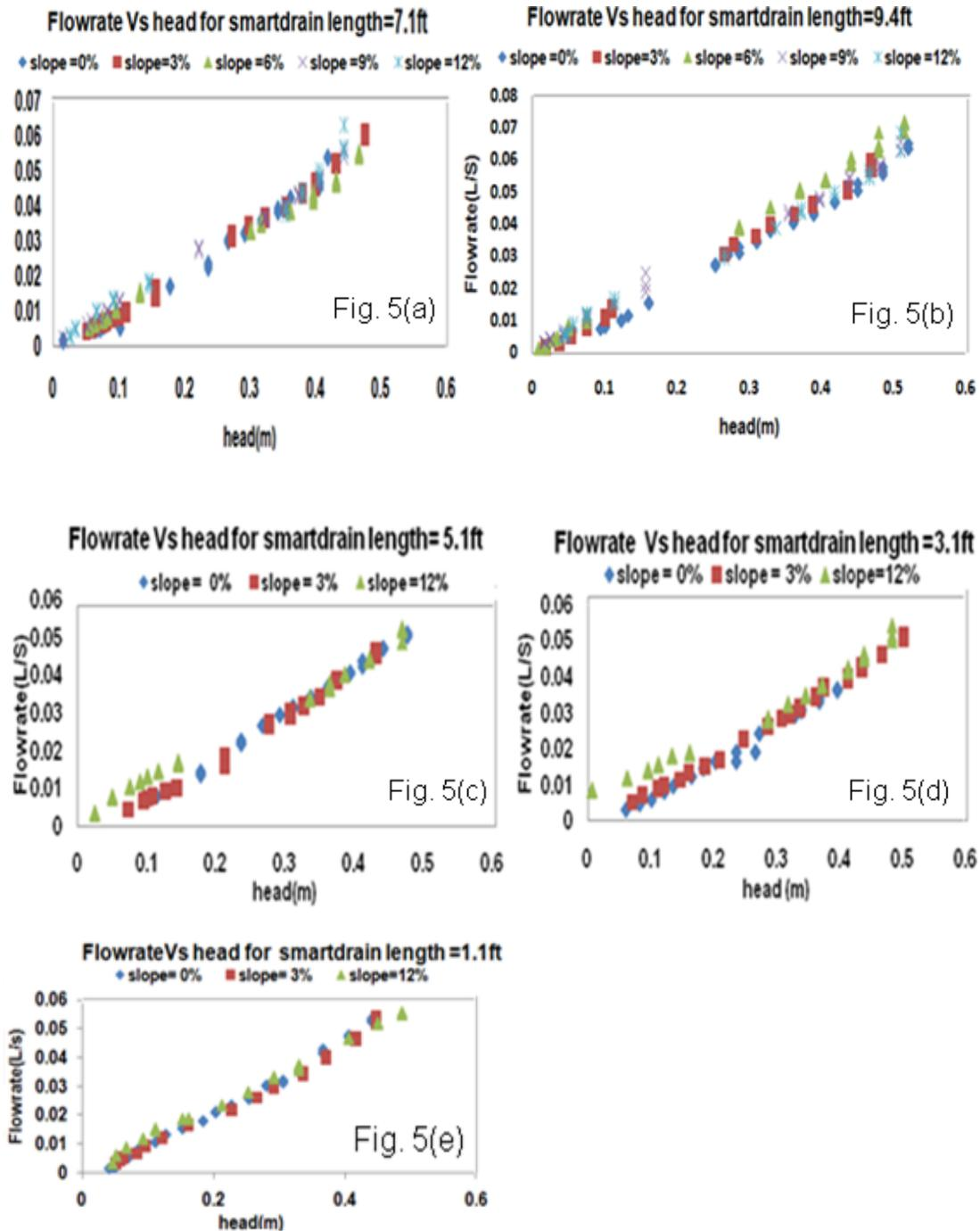
Figure 5, plots of flowrate versus head for five different SmartDrain™ length ( a to e) tested for five different slopes.
